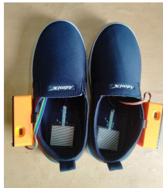
Fig 2: Working model of smart shoe
